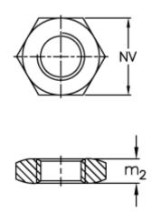
$\begin{array}{ll} m2 &= 10.0\\ Nominal size = M20\\ NV &= 30.00\\ Thread pitch = 2.50\\ Weight (g) &= 38.0 \end{array}$
